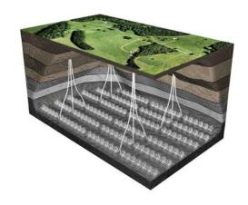
The drill rig and associated infrastructure can be removed from the site after the well is fractured, with only the gas / oil production and transmission infrastructure remaining. A single well could be expected to produce gas for up to 20 years.
